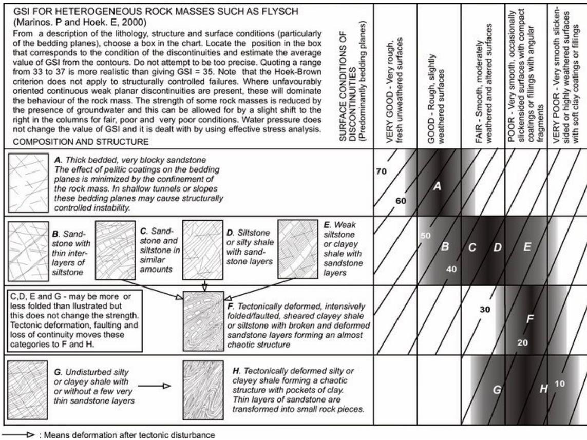
Figure 8: Geological Strength Index for heterogeneous rock masses such as flysch from Marinós and Hoek 2000.
