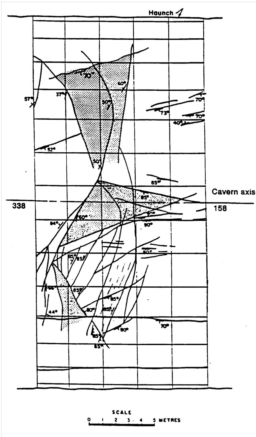
Figure 6: A plan of the traces of geological features mapped in part of the cavern roof. The shaded areas represent potentially unstable wedges requiring reinforcement.
