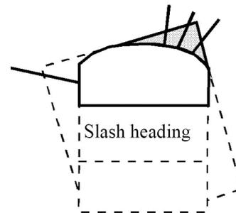
The margin sketch shows a support design which is based upon the largest possible wedges which can occur in the roof and walls of the excavation. These wedges can sometimes form in rock masses with very persistent discontinuity surfaces such as bedding planes in layered sedimentary rocks. In many metamorphic or igneous rocks, the discontinuity surfaces are not continuous and the size of the wedges that can form is limited by the persistence of these surfaces
