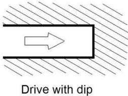
The value of  $A + B = 46$  and this means that, for joints of fair condition (slightly weathered and altered) and a moderate water inflow of between 200 and 1,000 gallons per minute, Table 3 gives the rating for  $C = 16$ . Hence, the final value of the rock structure rating  $RSR = A + B + C = 62$ .
