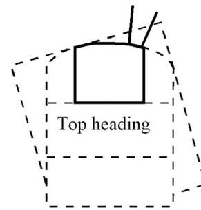
When dealing with large excavations of this type, the structural geology of the surrounding rock mass will have been defined from core drilling or access adits and a reasonable projection of potential wedges will be available. These projections can be confirmed by additional mapping as each stage of the excavation is completed. The program UNWEDGE provides an effective tool for exploring the size and shape of potential wedges and the support required to stabilise them.
