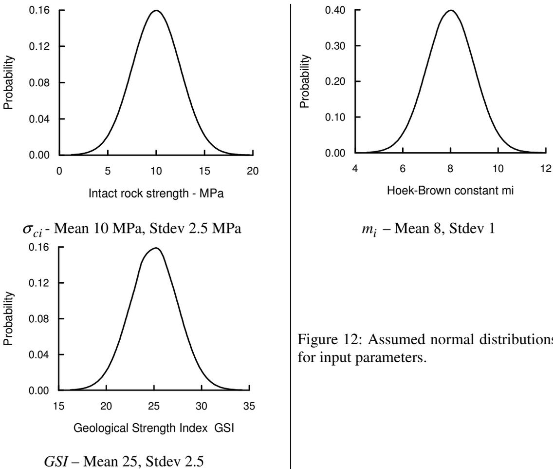
Figure 12: Assumed normal distributions for input parameters.
