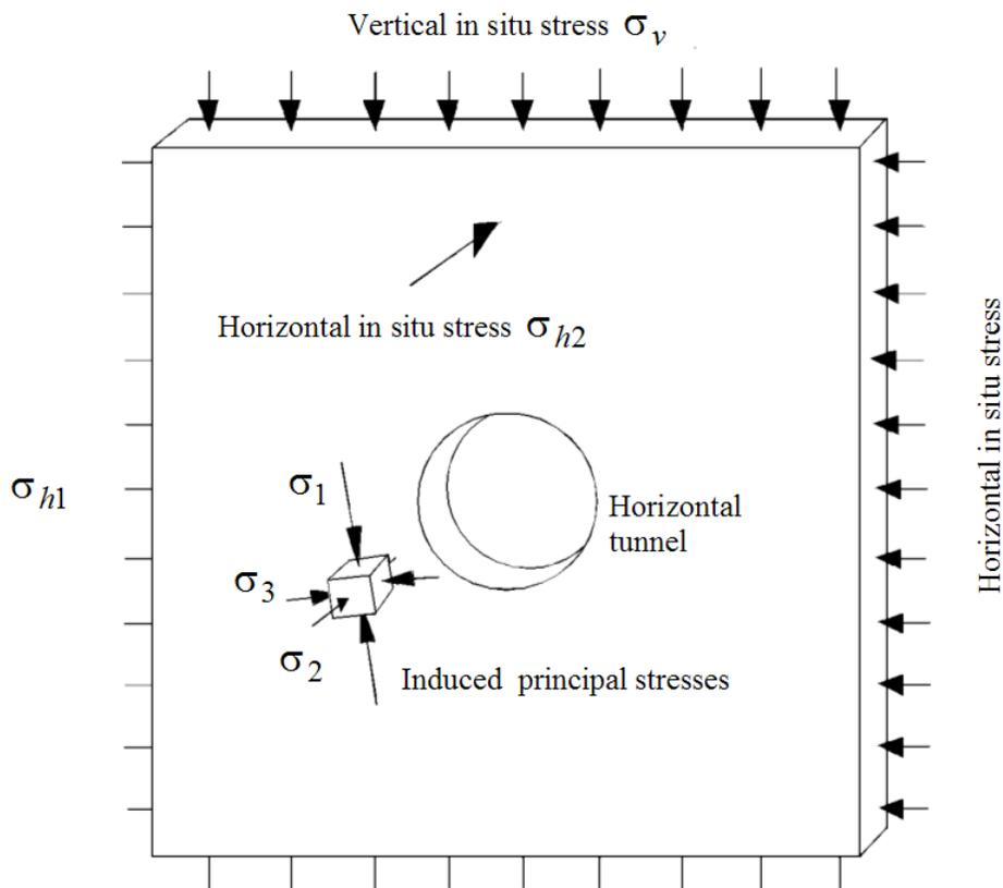
Figure 5: Illustration of principal stresses induced in an element of rock close to a horizontal tunnel subjected to a vertical in situ stress  $\sigma_v$ , a horizontal in situ stress  $\sigma_{h1}$  in a plane normal to the tunnel axis and a horizontal in situ stress  $\sigma_{h2}$  parallel to the tunnel axis.
