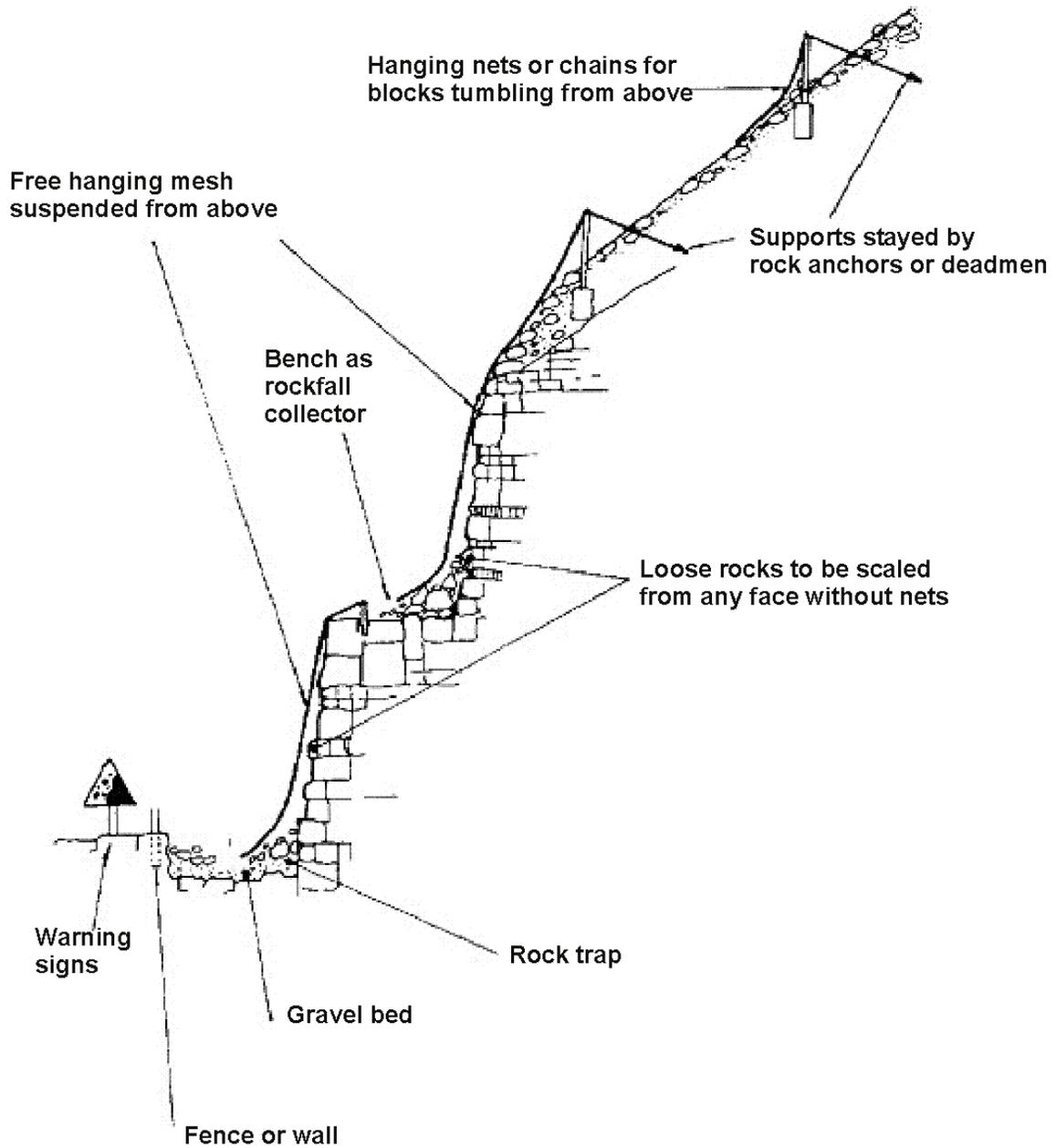
Figure 7: Rockfall control measures. After Fookes and Sweeney (1976).
