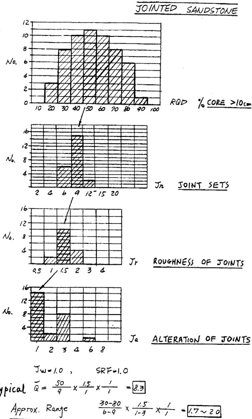
Figure 4: Histograms showing variations in RQD, J<sub>n</sub>, J<sub>r</sub> and J<sub>a</sub> for a dry jointed sandstone under 'medium' stress conditions, reproduced from field notes prepared by Dr. N. Barton.
