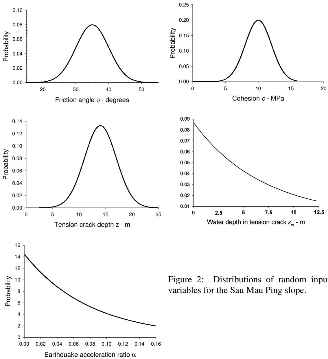
Figure 2: Distributions of random input variables for the Sau Mau Ping slope.
